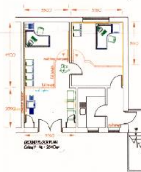
GROUND FLOOR CEILING PLAN Gallery Height - 2540mm
